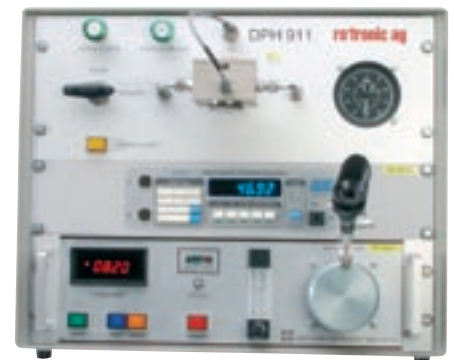
DPH 911 Reference dew point mirror for certification of SCS* humidity standards
